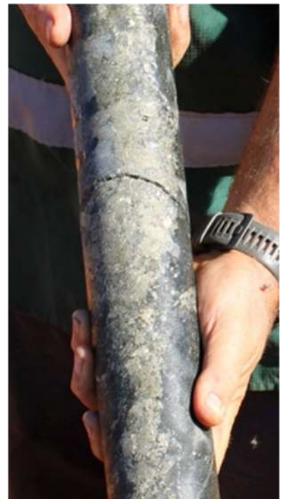
Figure 1: BHRCD018 core from 305.97m showing massive and blebby sulphide through altered Andesite/Gabbro
