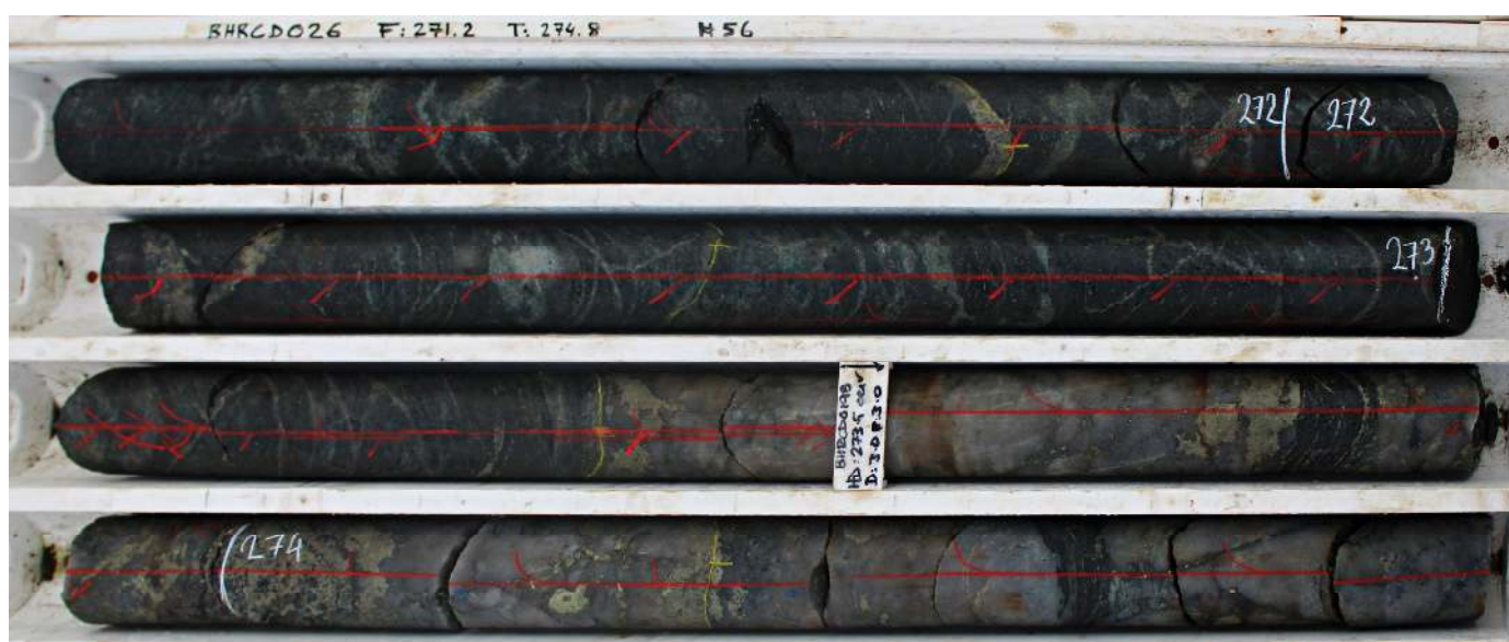
Figure 4: BHD026 core tray 56 from 271.2m-274.8m showing massive and blebby sulphides through quartz veining and altered Gabbro
