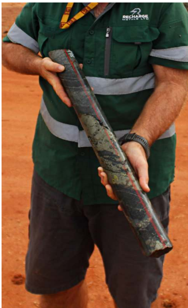
Figure 5: BHD026 core from 198 – 198.8m, showing blebby sulphides through altered ultramafic
