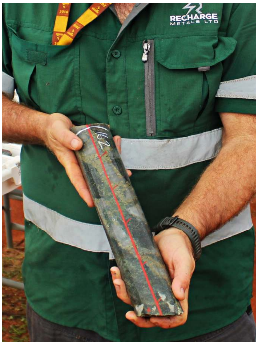
Figure 3: BHD026 core from 162-162.35.m, showing blebby sulphides through altered feldspar porphyry
